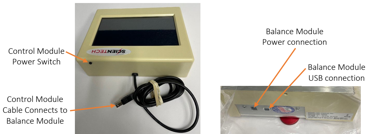
Figure 3. Control Module Power Switch & Balance Module Ports
